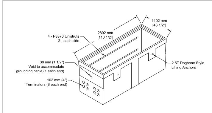
INSTALLATION INFORMATION MANUFACTURED IN ACCORDANCE WITH CSA A23.4 4 - 2.5T DOGBONE STYLE LIFTING ANCHORS
