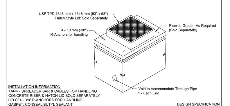
53" 53" [1346] [1346] Void to accommodate 76 mm [3"] Through Pipe - As Required 1702 mm 1899 mm [67"] [74 3/4"] As Required 102 mm Void to accommodate As Required [4"] Through Pipe
