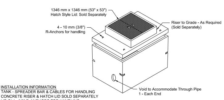
LID C/ 4 - 3/8" R-ANCHORS FOR HANDLING GASKET: CONSEAL BUTYL SEALANT
