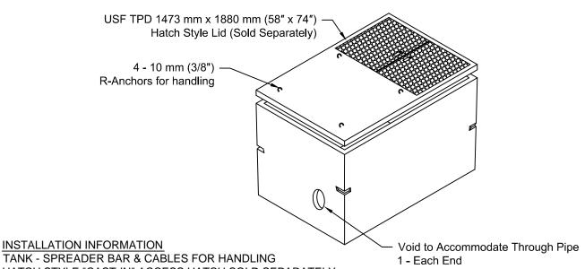
TANK - SPREADER BAR & CABLES FOR HANDLING
