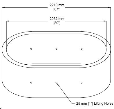
INSTALLATION INFORMATION 6 - 25 mm [1"] LIFTING HOLES WEIGHT: 2250 LBS / 1020 KG
