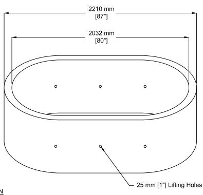
INSTALLATION INFORMATION 6 - 25 MM [1"] LIFTING HOLES WEIGHT: 1550 LBS / 680 KG
